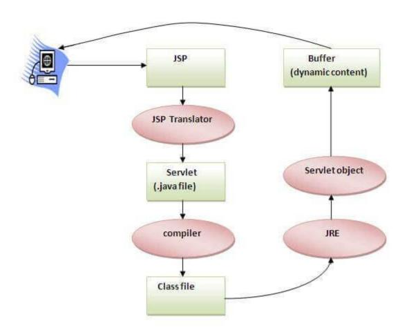
As depicted in the above diagram, JSP page is translated into Servlet by the help of JSP translator. The JSP translator is a part of the web server which is responsible for translating the JSP page into Servlet. After that, Servlet page is compiled by the compiler and gets converted into the class file. Moreover, all the processes that happen in Servlet are performed on JSP later like initialization, committing response to the browser and destroy.
