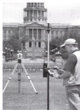
Robotic total station
