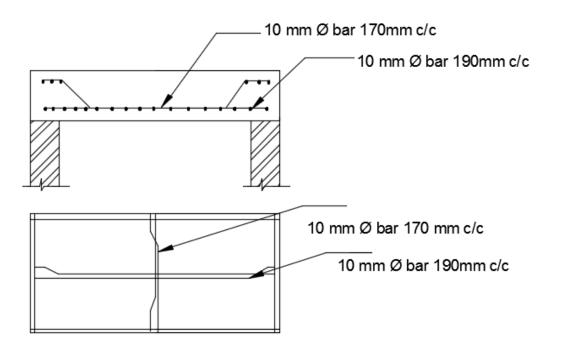
2.A slab has clear dimensions 3.5 m x 6 m with wall thickness 230 mm the live load on the slab is  $5 \text{ kN/m}^2$  and a finishing load of  $1 \text{kN/m}^2$  may be assumed. Using M20 concrete and Fe415 steel, design the slab
