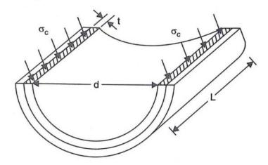
$\sigma_c$  = Compressive circumferential stress exerted by wire on cylinder =L $\times \frac{\pi}{2} \times d_w \times \sigma_w$
