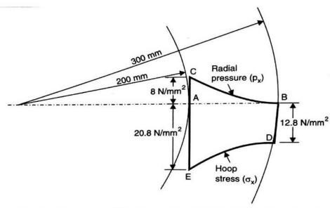
C is parabolic. The curve BC shows the variation of radial pressure across AB.
