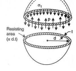
The stress  $\sigma_1$  is tensile in nature The fluid inside the shell is also having tendency to split the shell into two hemispheres along y-y axis. Then it can be shown that the tensile hoop stress will also be equal to  $\frac{pd}{4t}$ . Let the stress is  $\sigma_2$
