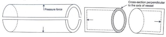
The forces, due to pressure of the fluid, acting at the thin cylinder, tend to burst the thin cylinder.
