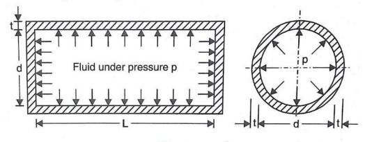
One of the internal pressure p, the cylindrical vessel may fail by splitting up in any one of the two ways.
