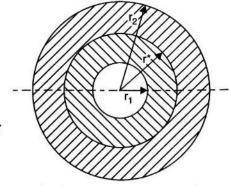
$p^*$  = Radial pressure at the junction of the two cylinders.
