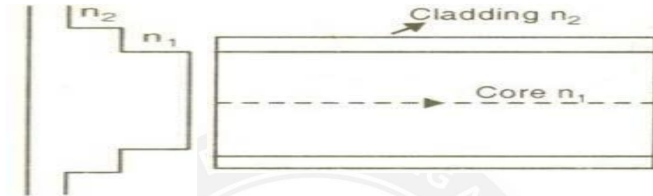
Fig 2.12.3 Step index fibre Single mode fibre
