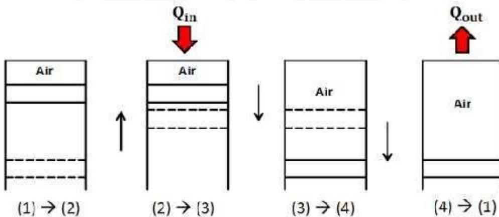
**Piston Position in Diesel Cycle Process**
