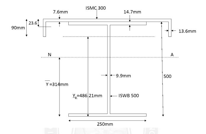
To find N.A of the section from bottom flange (tension)
