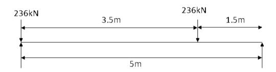
: Vertical shear due to wheel loads
