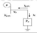
It is clear that  $V_F = Z_F I_F$ ,  $Vp(F) = V_F$  and  $Ip(F) = -I_F$
