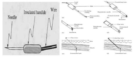
One of the main advantages of needle electrodes is that they are less susceptible to movement errors than surface electrodes.
