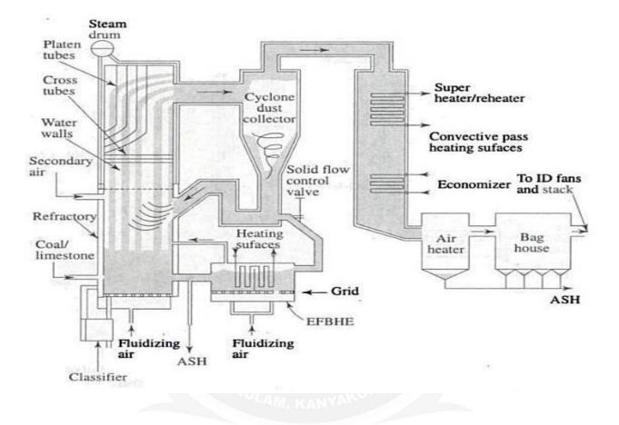
Schematic of a circulating fluidized bed boiler
