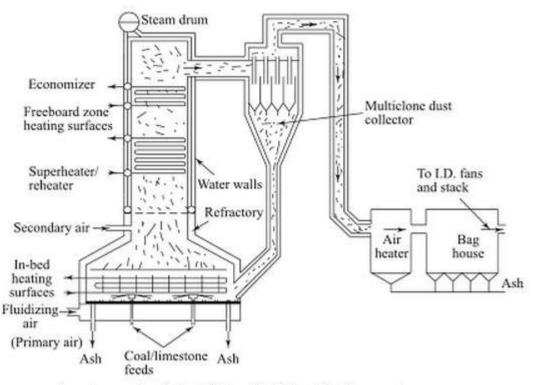
An atmospheric bubbling fluid bed boiler system
