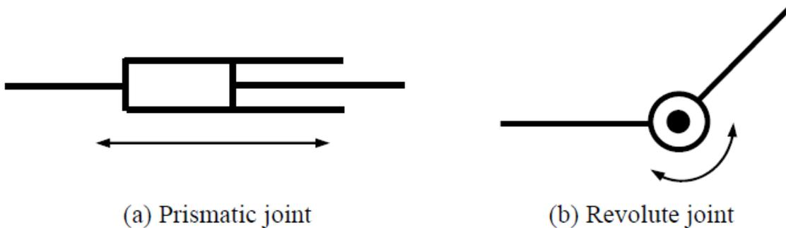
Combining these two types of primitive joints, we can create many useful mechanisms for robot manipulation and locomotion. These two types of primitive joints are simple to build and are well grounded in engineering design. Most of the robots that have been built are combinations of only these two types. Let us look at some examples.
