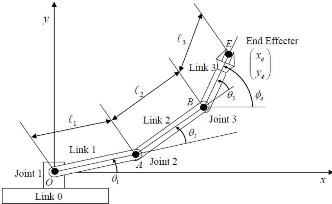
To describe this robot arm, a few geometric parameters are needed. First, the length of each link is defined to be the distance between adjacent joint axes. Let points O, A, and B be the locations of the three joint axes, respectively, and point E be a point fixed to the end-effector.
