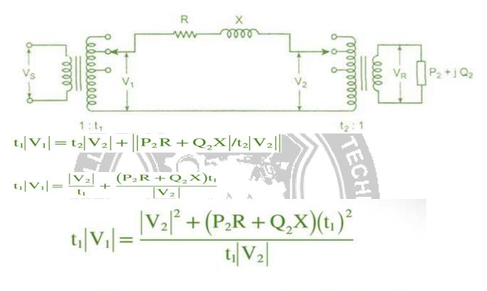
$$(t_1)^2 [|V_1||V_2| - (P_2R + Q_2X)] = |V_2|^2$$
