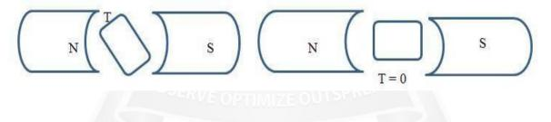
Figure 5.1.7 Rotor position due to revolving magnetic field [Source: "special electric machines" by Srinivasan page:1.3]
