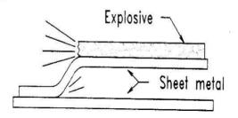
**Figure 5.1.7 Explosion bonding** [Source: "special electric machines" by Srinivasan page:1.3]
