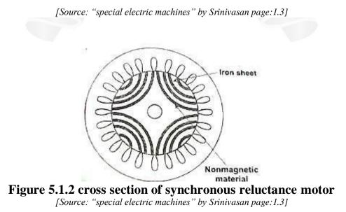
The rotor of the modern reluctance machine is designed with iron laminations in the axial direction separated by non-magnetic material. The performance of the reluctance motor may approach that of induction machine. With high saliency ratio a power factor oh 0.8 can be reached. The efficiency of a reluctance machine may be higher than an induction motor because there is no rotor copper loss. Because of inherent simplicity, robustness of construction and low cost.
