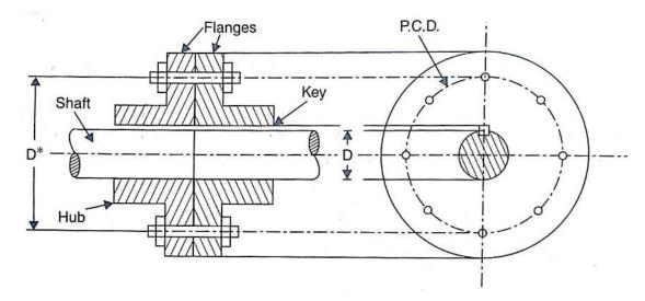
= Stress in bolt x Area of one bolt =  $q \times \frac{\pi \times d^2}{4}$
