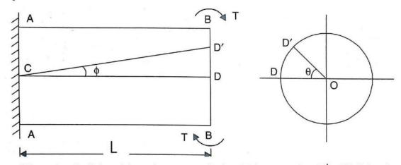
When the shaft is subjected to torque T then D is moved to  $D^l$ . If ' $\phi$ ' be the shear strain and ' $\theta$ ' be the angle of twist in length l then
