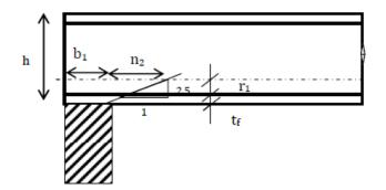
Problem1: Design a simply supported beam of span 5m carrying a reinforced concrete floor capable of providing lateral restraint to the top compression flange. The uniformly distributed load is made up of 20 KN/m imposed load and 20 KN/m dead load (section is stiff against bearing). Assume Fe 410 grade steel.
