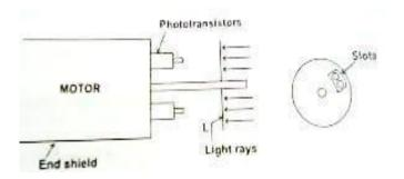
Figure 3.5.2 Optical position sensor [Source: "special electric machines" by R.Srinivasan page:4.11]
