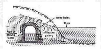
For maximum yield the galleries may be placed at full depth of the acquifer. Infiltration galleries may be constructed with masonary or concrete with weep holes of 5cm x 10cm.
