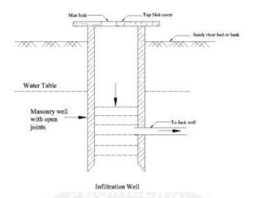
For the purpose of inspection of well, the manholes are provided in the top cover. The water filtrates through the bottom of such wells and as it has to pass through sand bed, it gets purified to some extent. The infiltration well in turn are connected by porous pipes to collecting sump called jackwell and there water is pumped to purification plant for treatment.
