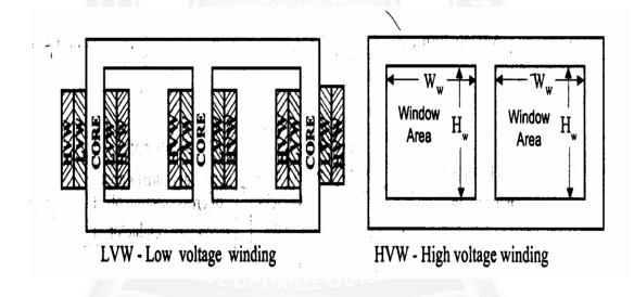
Figure 2.2.1 Core type three phase transformer
