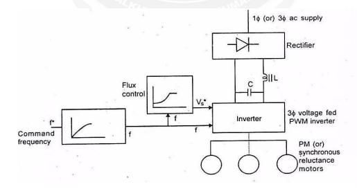
Figure 3.1.1 Separate Controlled Mode
