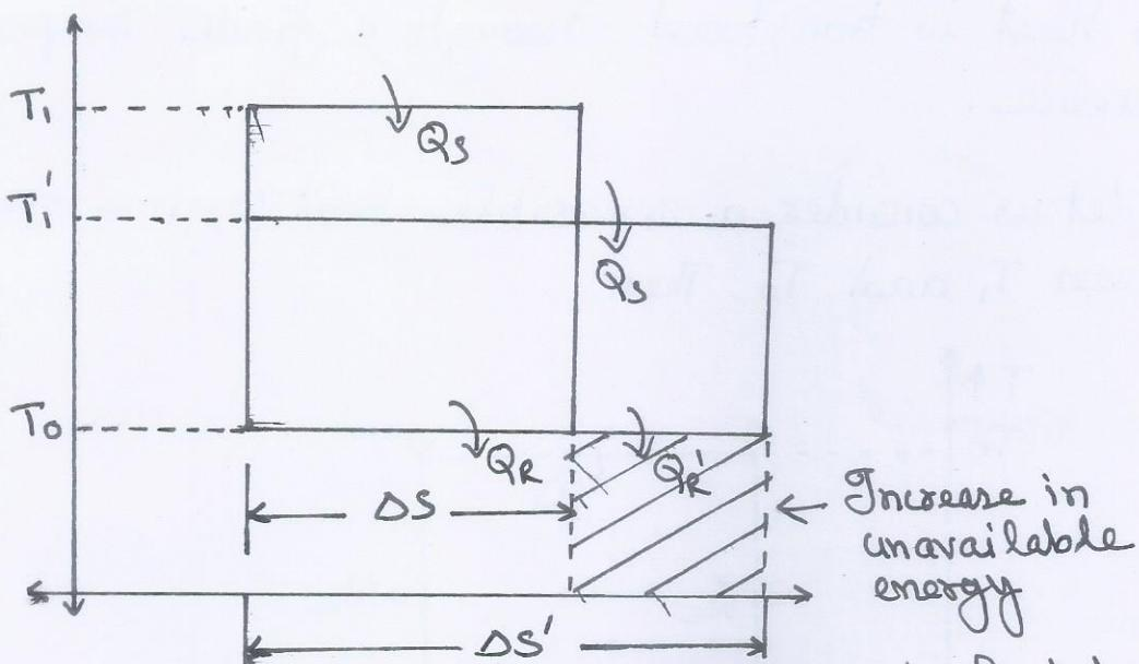
Increase in unavailable energy due to heat transfer through a finite temperature difference.
