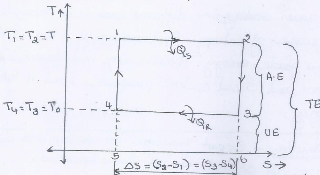
TE, AE and UE of a source on T-S diagram
