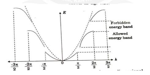
Fig5.14 Plot of energy Vs. wave vector in one dimensional lattice
