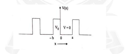
Fig. 5. 12 One dimensional periodic potential (Kronig and Penny model)
