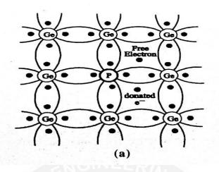
Fig 2.4.1 crystal structure-N type semiconductor
