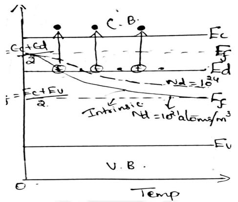
Fig 2.4.2-Variation of Fermi level with temperature
