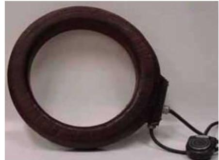
Also, flexible conductive cables can be wrapped around a component to form a coil. The number of wraps is determined by the magnetizing force needed and of course, the length of the cable. Normally, the wraps are kept as close together as possible. When using a coil or cable wrapped into a coil, amperage is usually expressed in ampere-turns. Ampere-turns is the amperage shown on the amp meter times the number of turns in the coil.
