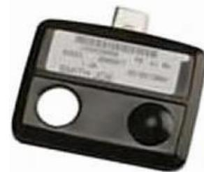
A *TLD* has a phosphor, such as lithium fluoride (LiF) or calcium fluoride (CaF), in a solid crystal structure. When a *TLD* is exposed to ionizing radiation at ambient temperatures, the radiation interacts with the phosphor crystal causing some of the atoms in the material to produce free electrons and become ionized. The free electrons are trapped and locked into place in the imperfections in the crystal lattice structure.
