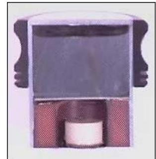
The thickness of the active element is determined by the desired frequency of the transducer. A thin wafer element vibrates with a wavelength that is twice its thickness. Therefore, piezoelectric crystals are cut to a thickness that is  $1/2$  the desired radiated wavelength. The higher the frequency of the transducer, the thinner the active element is.
