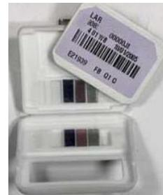
The major advantages of a film badge as a personnel monitoring device are that it provides a permanent record, it is able to distinguish between different energies of photons, and it can measure doses due to different types of radiation. It is quite accurate for exposures greater than 100 *mR*. The major disadvantages are that it must be developed and read by a processor (*which is time consuming*) and prolonged heat exposure can affect the film.
