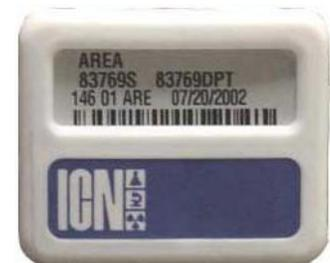
The film is contained inside a film holder or badge. The badge incorporates a series of filters to determine the quality of the radiation. Radiation of a given energy is attenuated to a different extent by various types of absorbers. Therefore, the same quantity of radiation incident on the badge will produce a different degree of darkening under each filter. By comparing these results, the energy of the radiation
