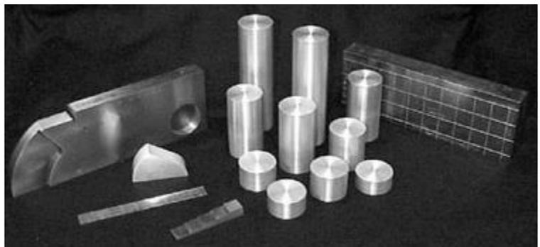
signal. By comparing the signal from the reference standard to that received from the actual flaw, the inspector can estimate the flaw size.
