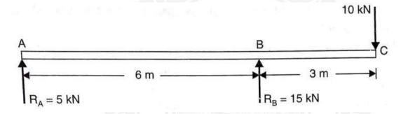
BM for the section X-X is given by,
