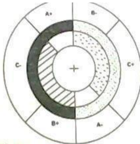
Figure 3.6.2 BLDC motor with 180° magnet arc and 120° square wave phase currents [Source: "special electric machines" by R.Srinivasan page:4.11]
