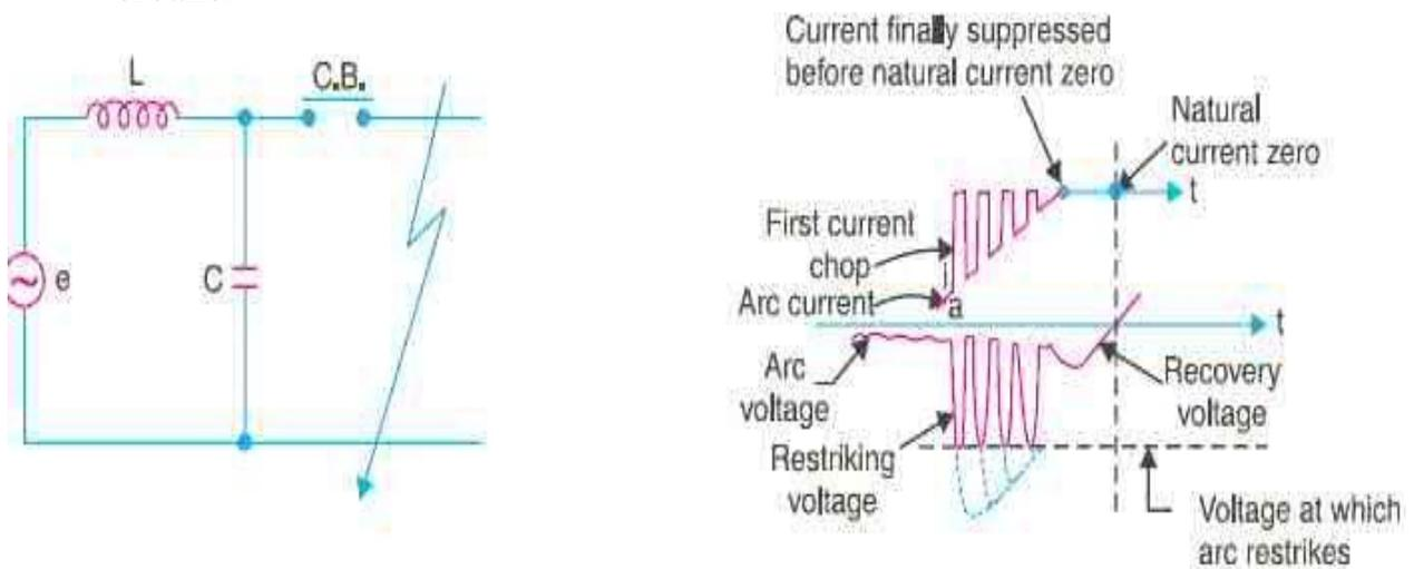
**Figure 5.6.1 Equivalent circuit and Characteristic of Current chopping**
