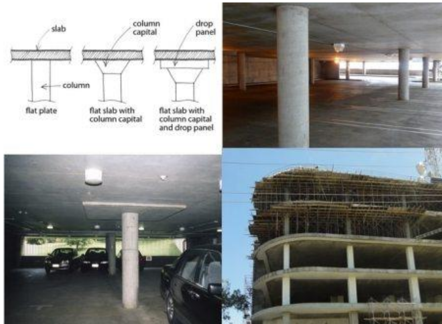
Fig.8: Flat slab and flat plate structure system
