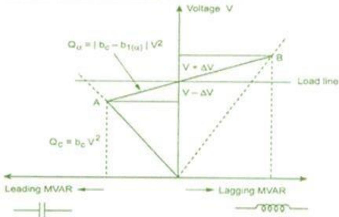
**Thyristor Switched Capacitor and Thyristor Controlled Reactor [TSC – TCR]**
