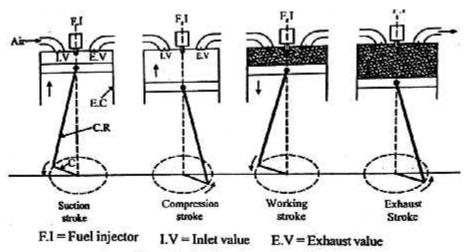
Four stroke diesel cycle engine
