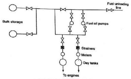
Fuel system for a diesel power plant
