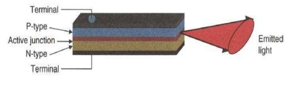
A LED is a p-n semiconductor device that emits light when a voltage is applied across its two terminals
