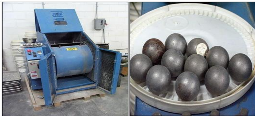
FIG.17 LOS ANGELES ABRASION TEST APPARATUS
