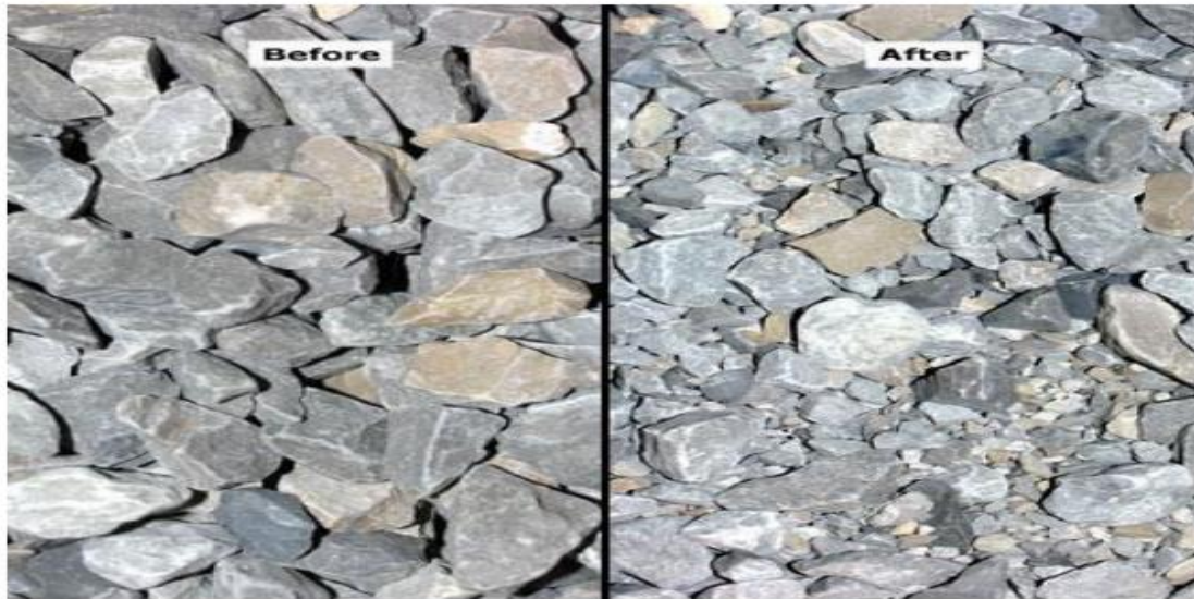
FIG.18 ABRASION OF AGGREGATES BEFORE AND AFTER ABRATION TEST
