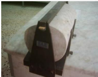
The jig for aligning concrete cylinder and bearing strips
