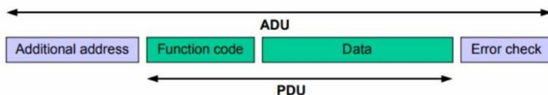
Figure 3: General MODBUS frame
