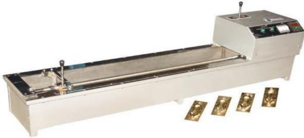
FIG. 20 DUCTILITY APPARATUS ON BITUMEN
