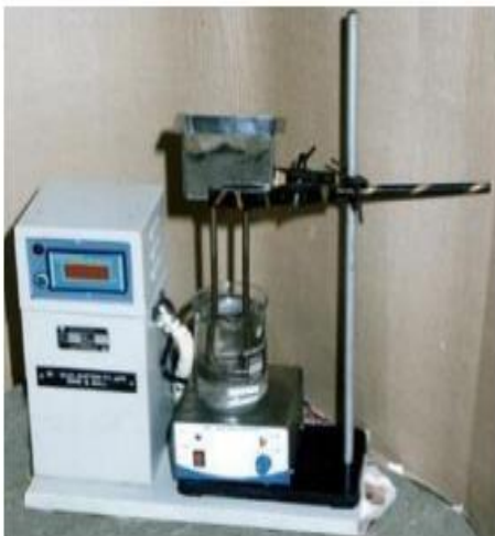
FIG. 22 SOFTENING POINT TEST APPARATUS ON BITUMEN
