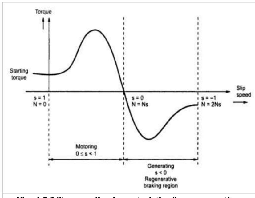
Fig. 4.5.3 Torque-slip characteristics for regenerative
