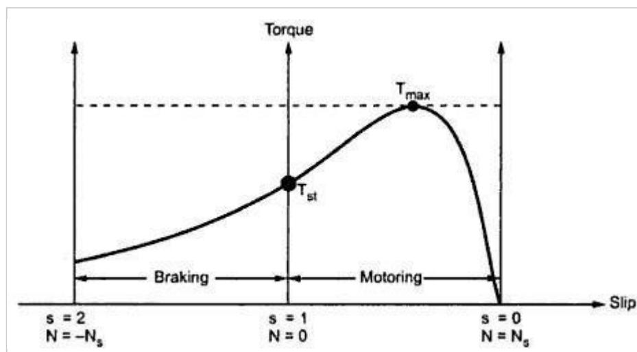
**Fig. 4.5.4 Torque-slip characteristics**
