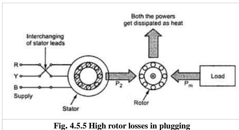
Fig. 4.5.5 High rotor losses in plugging
