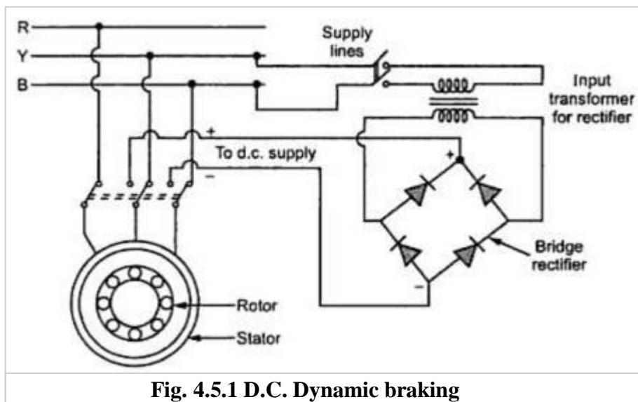
Fig. 4.5.1 D.C. Dynamic braking
