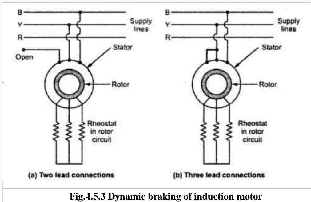
**Fig.4.5.3 Dynamic braking of induction motor**
