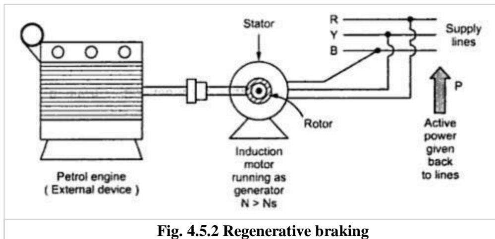
Fig. 4.5.2 Regenerative braking
