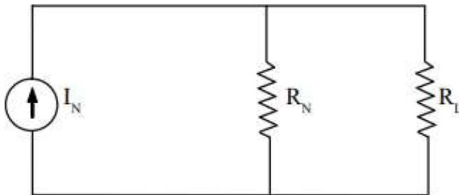
$$I_L = I_N \frac{R_N}{R_N + R_L} \quad \text{-----(8)}$$
