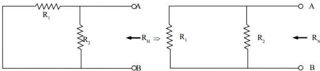
$$\therefore R_N = \frac{R_1 R_2}{R_1 + R_2} \quad \text{-----(7)}$$
