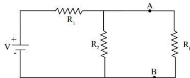
1. Replace  $R_L$  with a short circuit as in below figure
