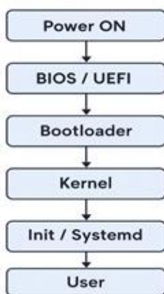
This diagram shows the **Linux Boot Process** – the sequence of steps that occur from when a computer is powered on until the user gets control of the system.
