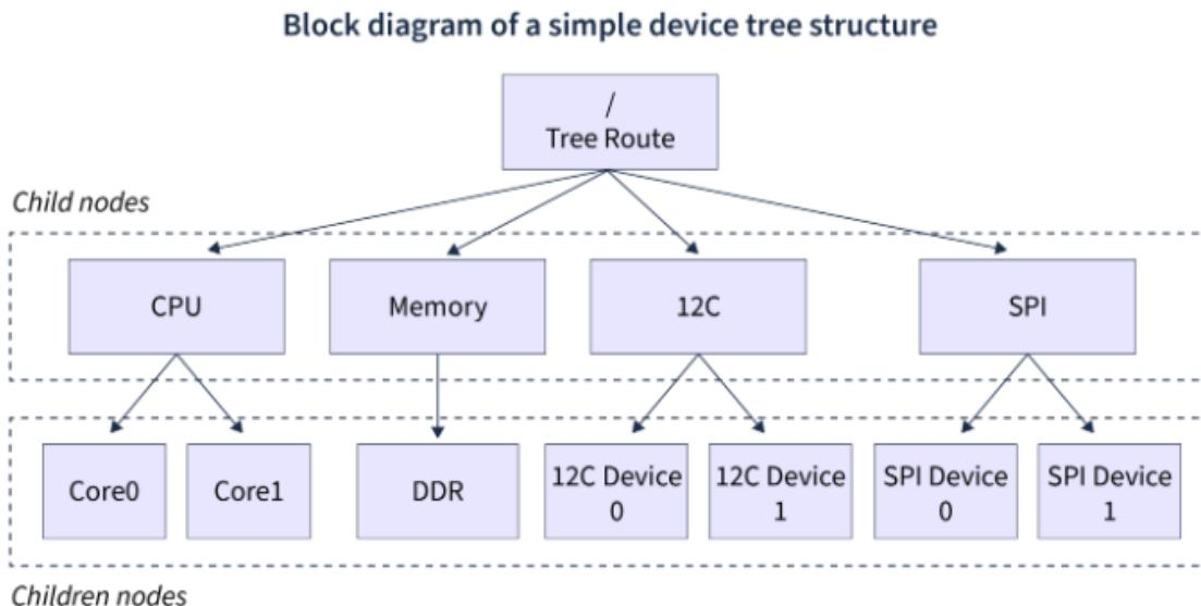
The above diagram is a **Block diagram of a simple device tree structure**.
