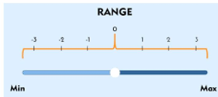
2. **Span:** Span is the difference between the maximum and minimum value of the measurement range.
