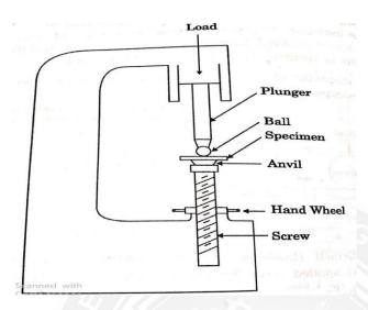
Brinell hardness test showing load, ball diameter, indented diameter and its thickness.
