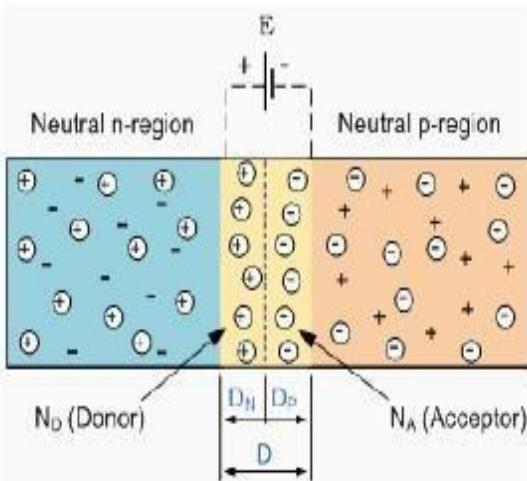
As the N-type material has lost electrons and the P-type has lost holes, the N-type material has become positive with respect to the P-type.
