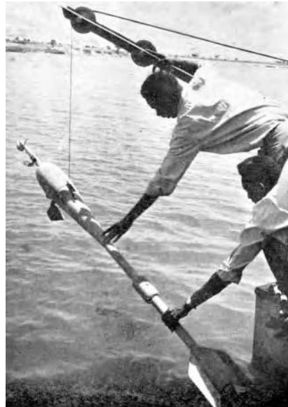
Fig. 10 Propeller-type Current Meter—Neyrtec Type with Sounding Weight
