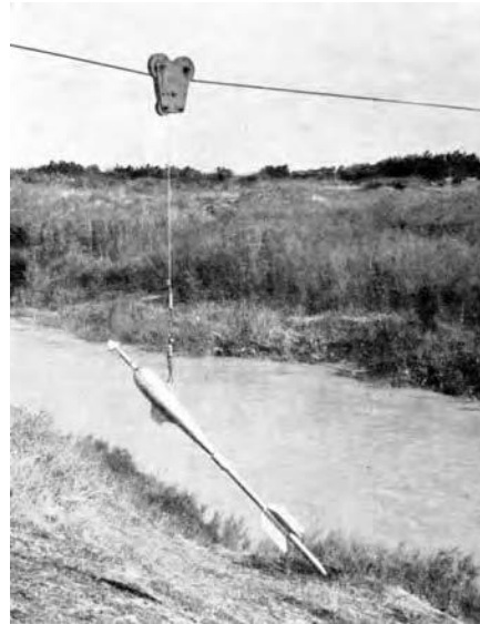
Fig. 12(b) Neyrtec Type Meter in a Cableway
