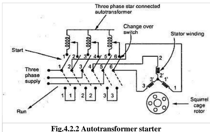
It consists of a suitable change over switch.
