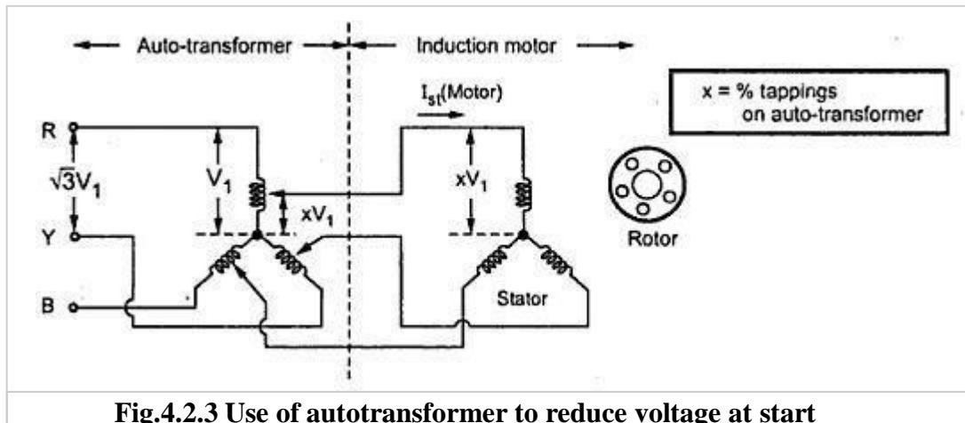
Fig.4.2.3 Use of autotransformer to reduce voltage at start
