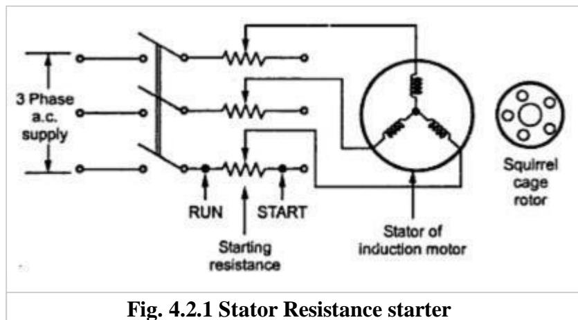
When the motor starts running, the resistances are gradually cut-off from the stator circuit. When the resistances are entirely removed from the stator circuit i.e. rheostats in RUN position then rated voltage gets applied to the stator. Motor runs with normal speed.
