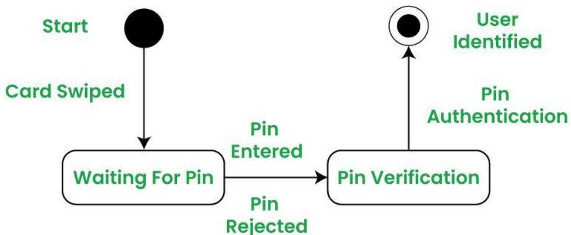
The State Machine Diagram above shows the different states in which the verification sub-system or class exists for a particular system.
