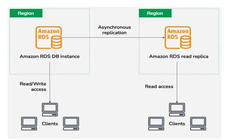
This configuration provides a resilient solution to scale applications globally while ensuring data redundancy and improved fault tolerance
