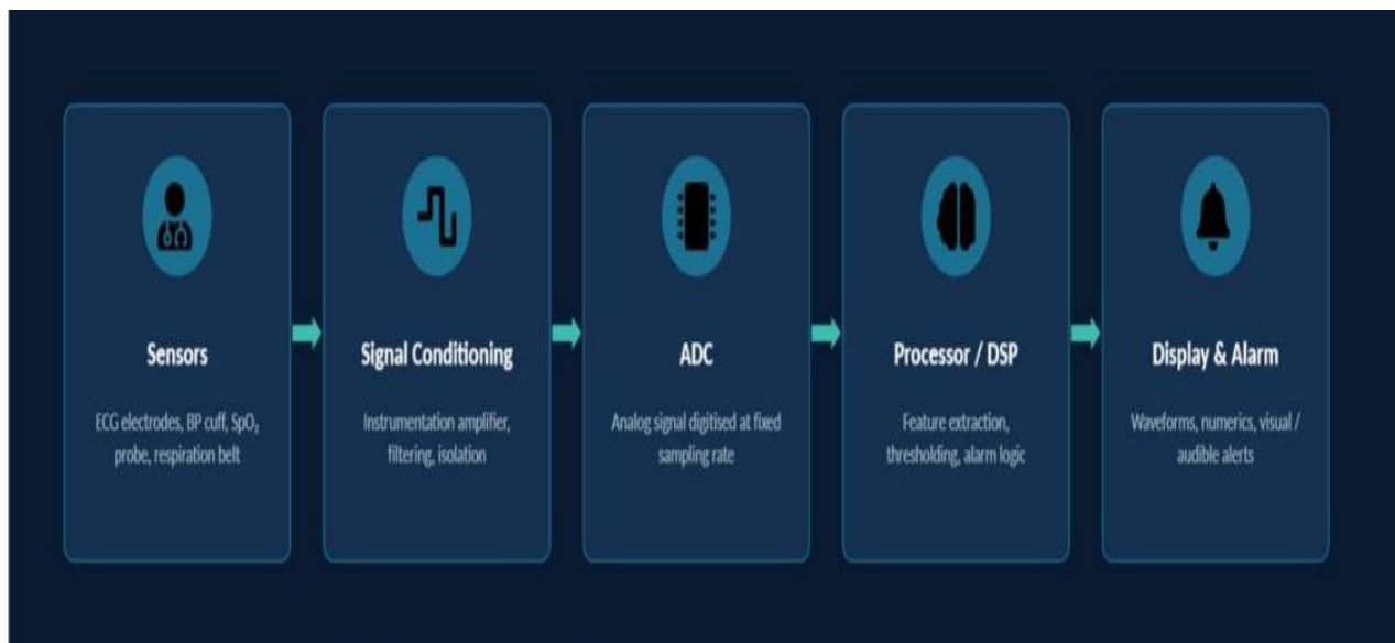
Fig 7.1 — General MPM signal chain from sensors to central monitoring station (Sensors: ECG electrodes, BP cuff, SpO 2 probe, respiration belt → Signal Conditioning: instrumentation amplifier, filtering, isolation → ADC: analog signal digitised at fixed sampling rate → Processor/DSP: feature extraction, thresholding, alarm logic → Display & Alarm: waveforms, numerics, visual/audible alerts; parallel network feed to Central Monitoring / EHR Station)
