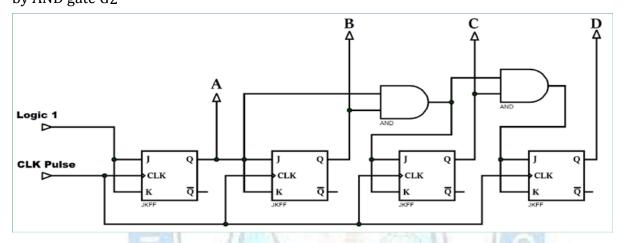
**Bit Synchronous Binary Counter**
