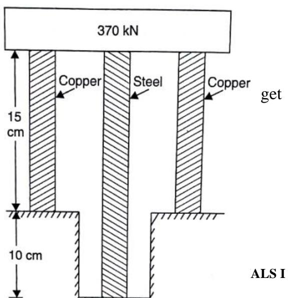
figure. The cross sectional area of steel rod is  $2500 \text{ mm}^2$  and of each copper rod is  $1600 \text{ mm}^2$ . Find the stresses in the rods. Take  $E$  for steel =  $2 \times 10^5 \text{ N/mm}^2$  and for copper =  $1 \times 10^5 \text{ N/mm}^2$ .
