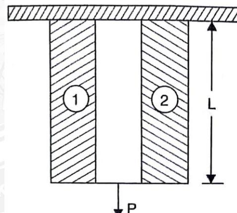
Now the total load on the composite bar is equal to the sum of the load carried by the two bars
