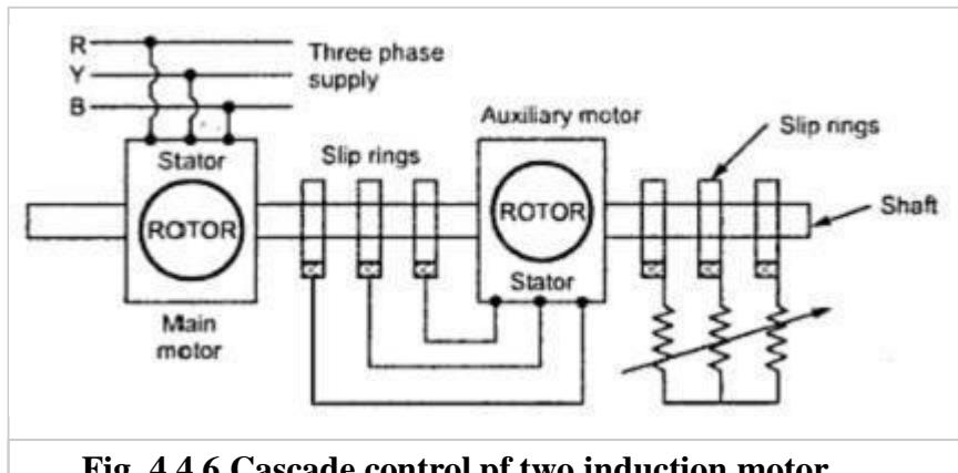
Fig. 4.4.6 Cascade control of two induction motor
