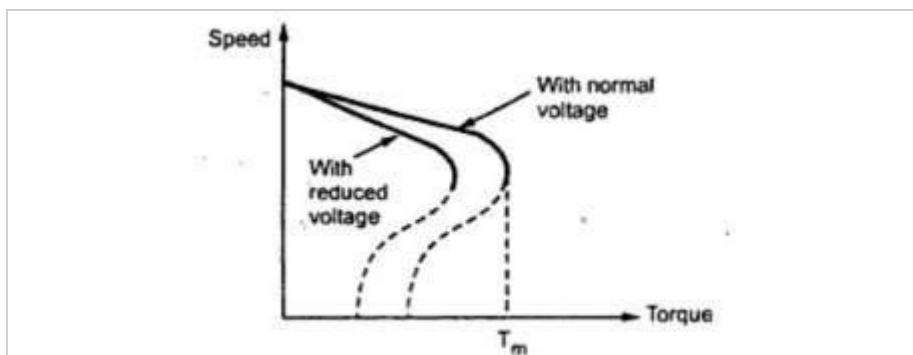
**Fig.4.4.3 Speed-torque curves for motor with voltage control**
