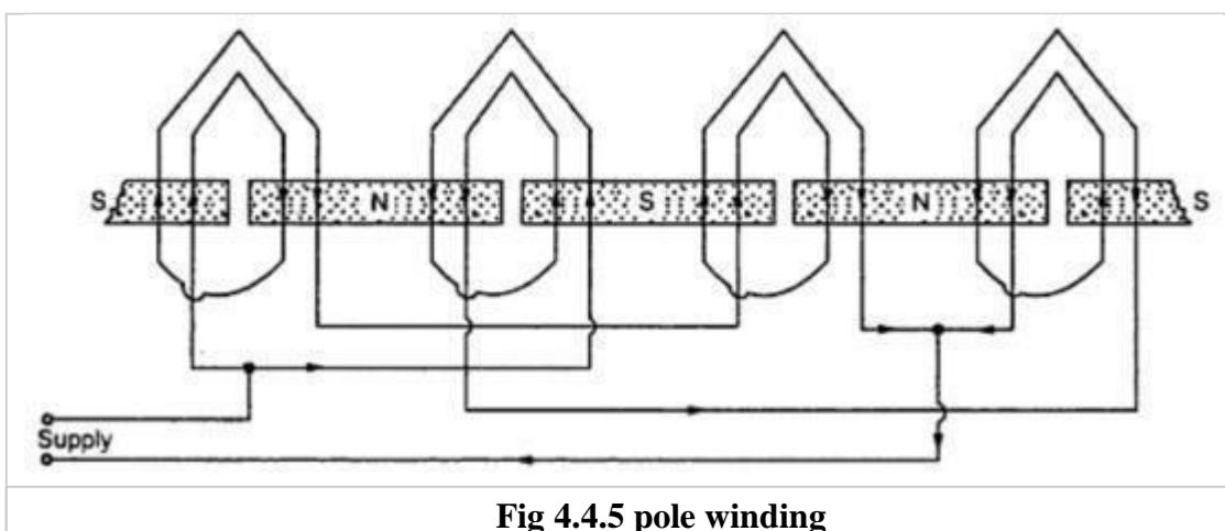
**Fig 4.4.5 pole winding**
