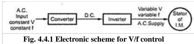
Fig. 4.4.1 Electronic scheme for V/f control
