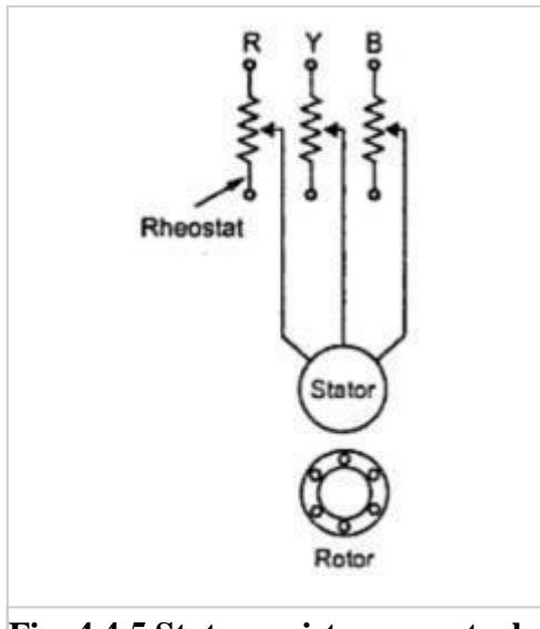
Fig. 4.4.5 Stator resistance control
