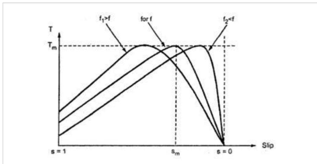
Fig. 4.4.2 Torque-slip characteristics with variable f and constant (V/f)
