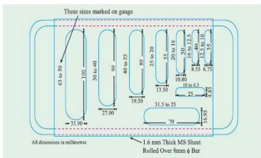
**Dimensions of Thickness and Length Gauges (IS: 2386 (Part I) – 1963****3. Test for Determination of Elongation Index :**
