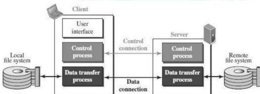
The above figure shows the basic model of the FTP.
