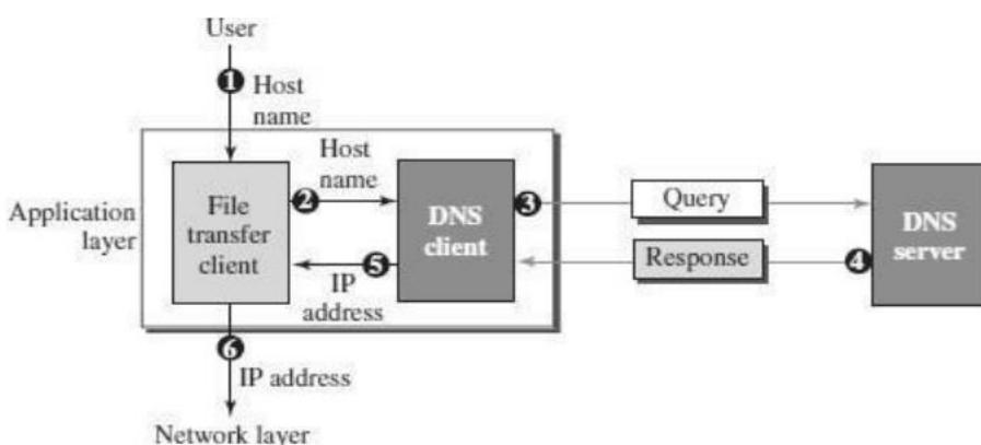
The following six steps shows the working of a DNS. It maps the host name to an IP address:
